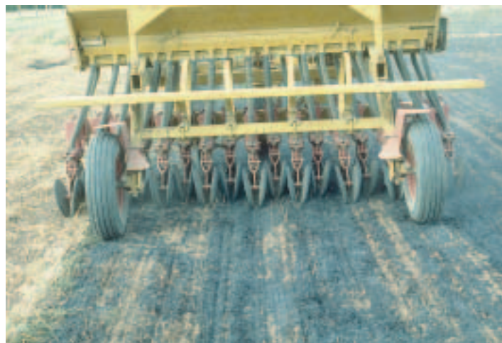
FIGURE 2. Planting no-till alfalfa into burned wheat stubble in August.
